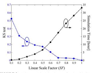
**FIGURE 3** K-S tests and simulation times as a function of the SF. The K-S tests agree when SF > 0.7, and the simulation time of SF = 0.7 is reduced to 52.6% compared to SF = 1. [Color figure can be viewed at wileyonlinelibrary.com]
