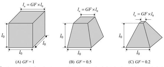
**FIGURE 5** The target geometries for a cube and two trapezoidal hexahedrons are described. The baselines and heights are retained as  $l_0$ , while  $l_u$  is determined by the GF
