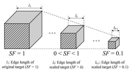
FIGURE 1 Original and downscaled target cubes. SF varies from 1 to 0.1 by a step of -0.1
